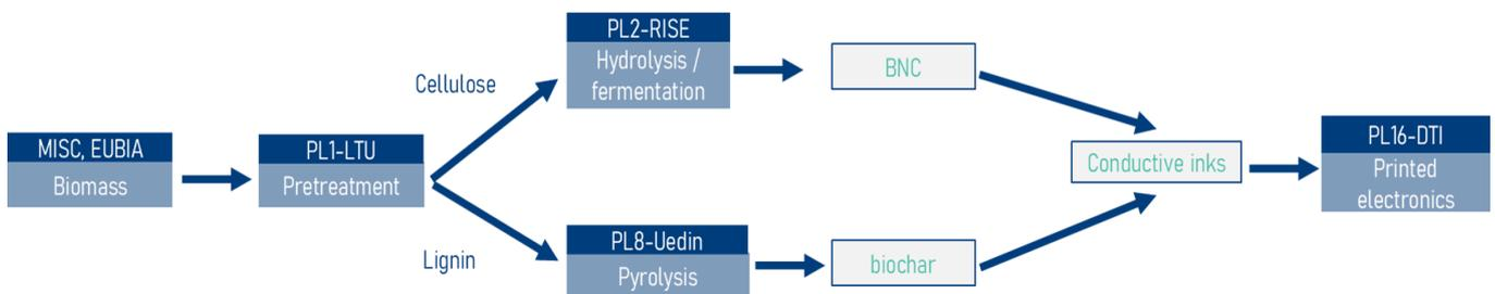
Figure 4: Process flow for the production and use of BNC and biochar
