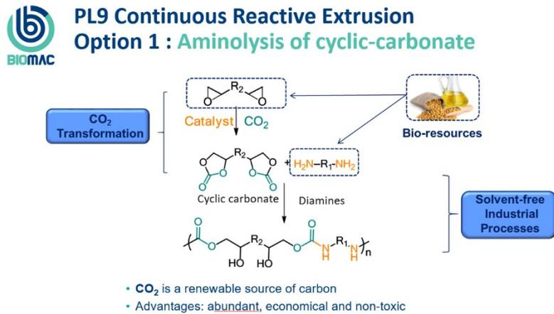
Figure 5: First approach evaluated to synthesize biobased NIPUs: step-growth polyaddition of cyclic dicarbonates and diamines.
