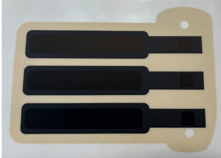
Figure 9: Picture of a product, consisting of 3 layers of ATR-136 and 3 layers of BC80 screen printed on BPUS.
