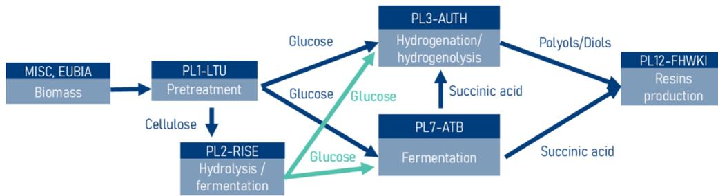
Figure 2: Process flow for the diols and succinic acid used by PL12 in the production of PUDs.
