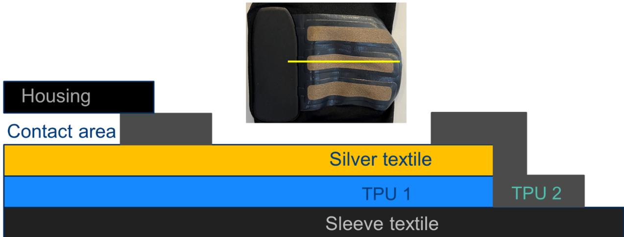
Figure 1: Picture of the EMG electrode part of MLI ELBOW, and a schematic of the design along a line indicated on the picture. TPU (Thermoplastic PolyUrethane) is a highly stretchable polymer.
