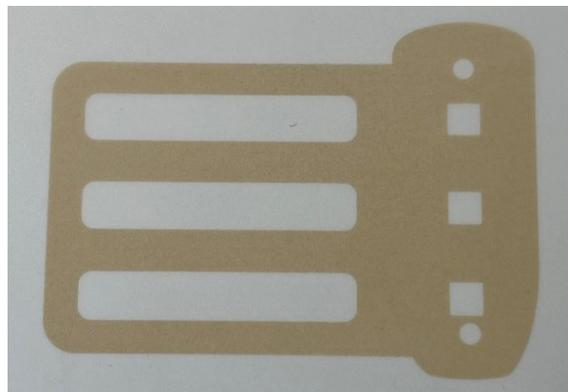
Figure 8: Picture of a single layer print of BC80 on a transfer substrate.
