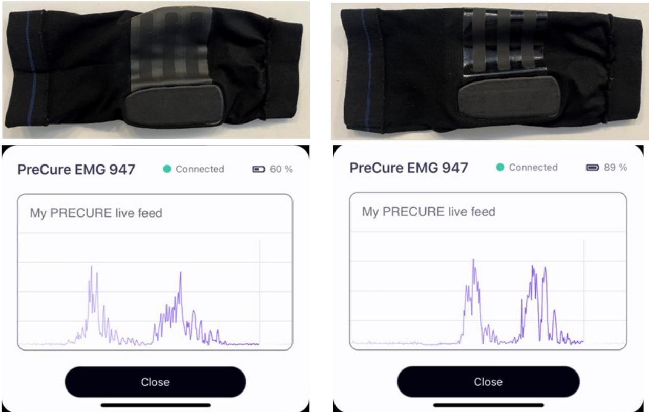
Figure 11: Pictures of prototypes at the top, and pictures of EMG measurements from PRECUREs app below. P8 is to the left and P9 to the right.
