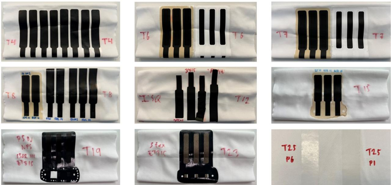
Figure 10: Pictures of samples used in wash durability testing. Pictures taken after 15 wash cycles.
