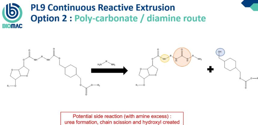
Figure 6: First approach evaluated to synthesize biobased NIPUs: step-growth polycondensation of polycarbonates and diamines
