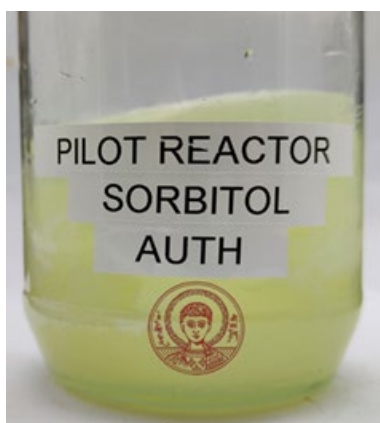
Sorbitol from the catalytic hydrogenation (PL3) of glucose hydrolysates.
