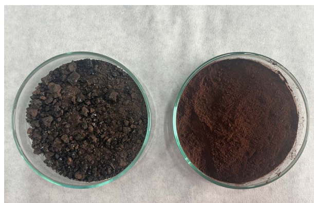
Figure 1: Organosolv lignin before (left) and after (right) 1h ball milling and 4h US treatment in water.
