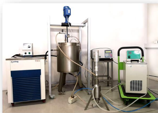
Ultrasonication equipment of Pilot Line 4
