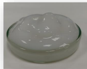
Nanocellulose obtained by a continuous process in BIOMAC
