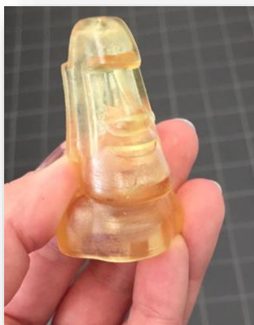
3D-printed biobased resin developed at PL12
